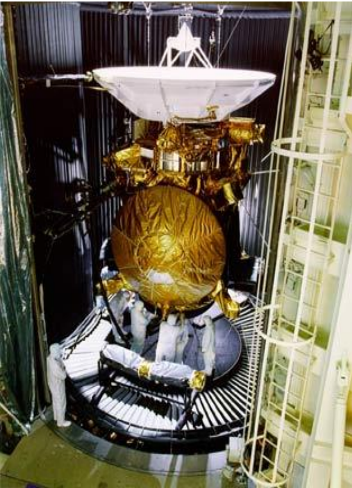
Cassini/Huygens by NASA / ESA to explore Saturn and Titan (initiated 1986) 6.7 m height / Ø 4 m launch mass: 5.82 t
