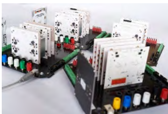
Figure 10 Flat-Sat Setup for easy Test & Development of Satellite Subsystems
